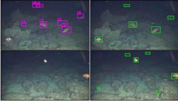
Figure 6. Comparison with an underwater fish detection network based on YOLO topology. [Left] Results of YOLO. [Right] Our results. Generally our algorithm provides better recall rate with less false positives.
